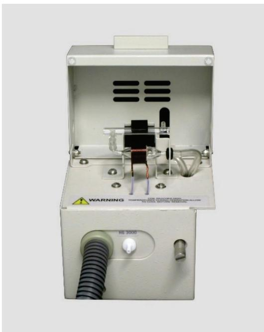
**Figure 2: Detail of the MC3000 showing the inductively heated trap and the optical cell**
